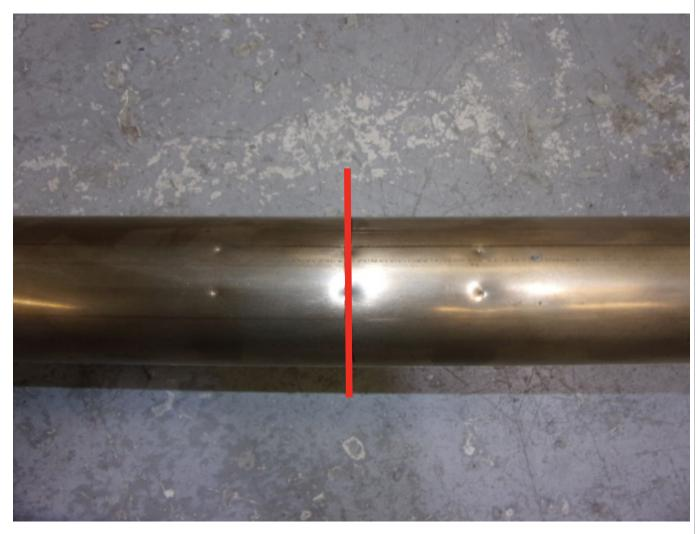
To make it easier to cut the exhaust we reccomend removing it from the car. Find the 3 pairs of indents and use the middle pair to mark out the cutting line. Cut along the line and de-bur the edges. Re-fit the original GPF and fit the Scorpion GPF-back following the line diagram above. NOTE: If fitting at the same time as our GPF-back system you won't need to cut the original system.
